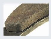
**Separation of the brake pad** The brake pad is partially separated from the base plate
