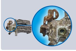
Internal oxidation. Brake piston seized up Sleeve damaged
