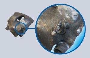
Guide bushing damaged
