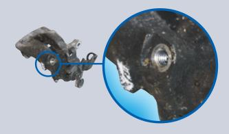
Housing damaged, spring mounting broken off
